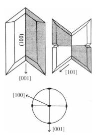
**Fig. 5.** The dovetail twin of gypsum. On the left the most frequent form consisting of two individuals; on the right the rare form with four individuals, displaying the orthorhombic composite symmetry. The two orientation states are distinguished by shading (after Hahn-Klapper (2003) with the permission of the IUCr).
