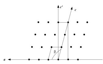
**Fig. 10.** A monoclinic *P* cell with  $c \cos \beta = -a/3$ , and the corresponding triple orthorhombic supercell projected parallel to the monoclinic axis  $\boldsymbol{h}$ .
