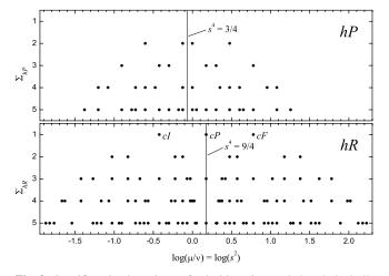
**Fig. 9.** Specific misorientations of primitive (hP) and rhombohedrally centred (hR) hexagonal lattices with multiplicity (twin index)  $\Sigma \leq 5$  as a function of the axial ratio s. Notice that the three types of cubic lattices appear as special cases of rhombohedral lattices.
