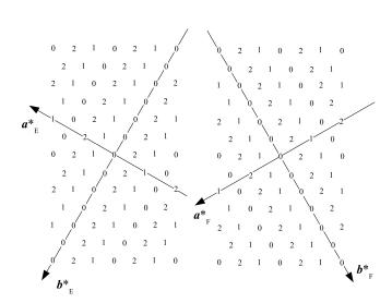
**Fig. 14.** Projection parallel to  $c^*$  of the monoclinic *C*-centred lattice with the metric in the a-c-plane as shown in Fig. 10, in six orientations differing by  $n \times 60^{\circ}$  rotations about  $c^*$ . Symbols have the same meaning as in Fig. 12.
