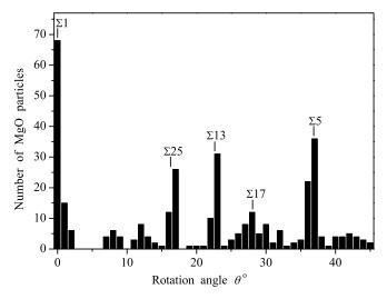
**Fig. 6.** Histogram of the number of MgO cubes in  $1^{\circ}$  intervals of the rotation angle  $\theta$  about  $\langle 001 \rangle$  for MgO smoke particles on a  $\{001\}$  surface of MgO.
