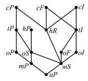
**Fig. 3.** The relation between the various Bravais types of lattices. The Bravais type at the upper end of a line is a special case with point group of higher order of the one at the lower end.
