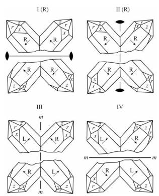
**Fig. 4.** The four variants of Japanese twins of quartz. The twin elements 2 and m are shown. In an actual twin either the upper or the lower part is realized. R, L: right-, left-handed quartz. The arrow gives the polarity of the twofold axis parallel to the plane of the drawing. The cases I(L) and II(L) are not shown. (reproduced from Hahn-Klapper (2003) with the permission of the IUCr).
