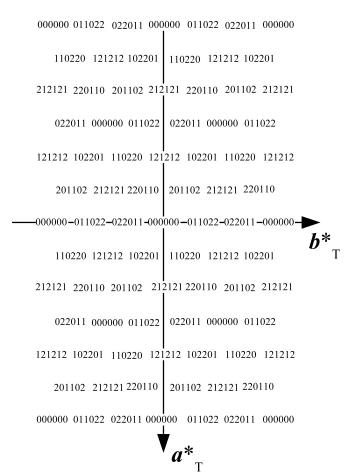
**Fig. 15.** Overlap of the six lattices in Fig. 14. Each sequence of six numbers corresponds to a row of nodes of  $\mathbf{L}^*_T$  with the same hk values. The six numbers give the corresponding value of  $l \pmod{3}$  for the 6 individuals.
