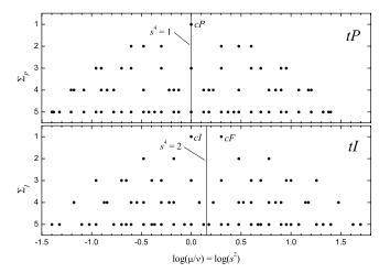
**Fig. 8.** Specific misorientations of primitive (tP) and body-centred (tI) tetragonal lattices with multiplicity (twin index)  $\Sigma \leq 5$  as a function of the axial ratio s. Notice that the three types of cubic lattices appear as special cases of the tetragonal types: cP as a special case of tP, cI and cF as special cases of tI.
